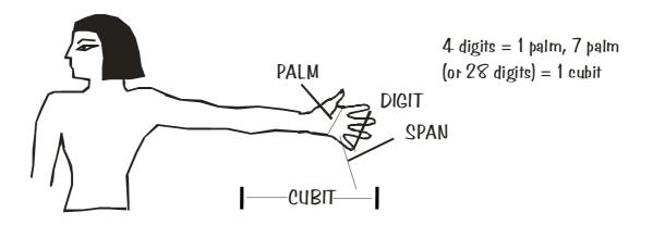
The Egyptians used a knotted rope to indicate the agreed length of a cubit. The ROYAL CUBIT (52.4cm) was used the most but the SHORT CUBIT (44.9cm) was also used.
